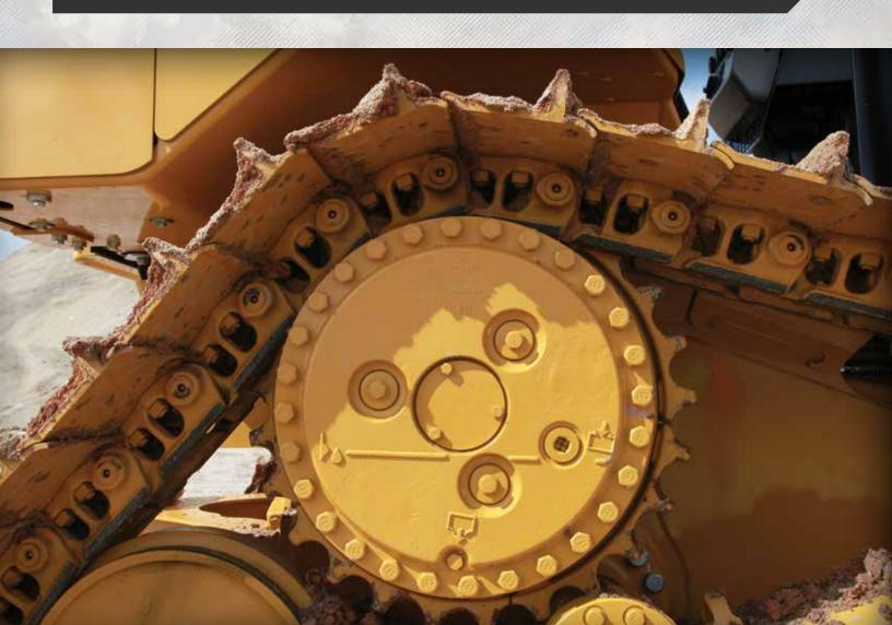
HDXL utilizes Positive Pin Retention 2 (PPR2) technology to extend undercarriage life. PPR2 mechanically locks the link to the pin to resist pin walking and link cracking for reliable sealing and track life. That means more uptime for your machine – and more productivity for your business.
